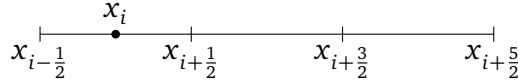
Figure 4: Reconstruct u_x(x_i, t_j) using only values at x_{i-1/2} , x_{i+1/2} , x_{i+3/2} and x_{i+5/2}
