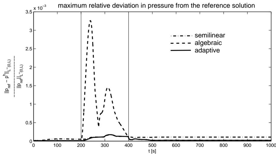
Figure 6: maximum relative deviation in the pipe from the reference solution per time step
