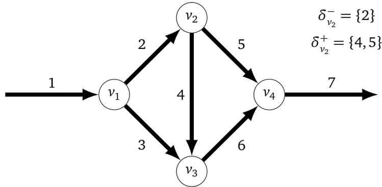
Figure 1: A small network; the ingoing pipes of node  $v_2$  are  $\delta_{v_2}^- = \{2\}$  and the set of outgoing pipes is  $\delta_{v_2}^+ = \{4, 5\}$
