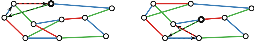
Fig. 1. A regular graph with two different starting locations. By following the color sequence “green, blue, red”, the agent either moves on a cycle (left) or not (right), but there is no way to distinguish between these two cases as vertices are indistinguishable. (Color figure online)
