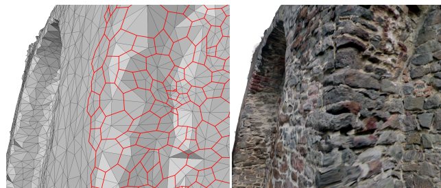
Figure 1: Left: Citywall triangle mesh with a portion of the resulting MRF (edges) overlaid in red. Right: Textured result. This dataset's size and structure stresses the need for an efficient, parallel solver without a restriction to regular grid-based topologies.
